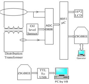
Fig. 3. The hardware structure for the ZIGBEE based transformer protection
