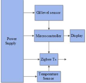
Fig 1. Block diagram of the end device
