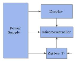
Fig.2. Block diagram of the coordinator unit
